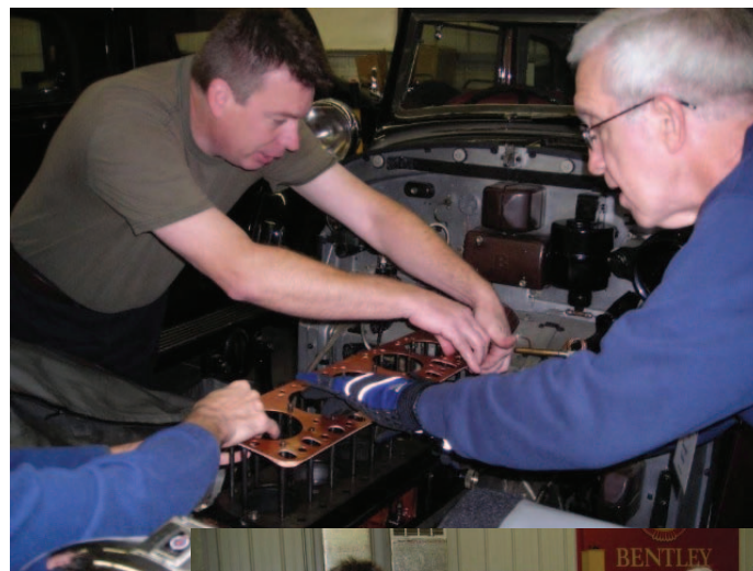
Top: Tim Jayne (l) and George Kalin install new head gasket.
