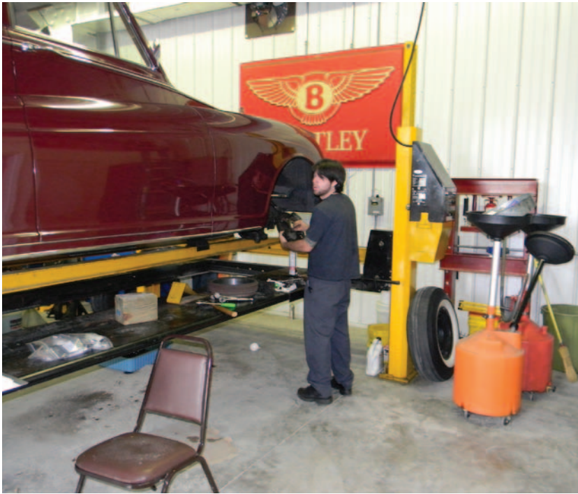
One of Palma's techs, John LeFlam, installing the right front brake cylinders.
